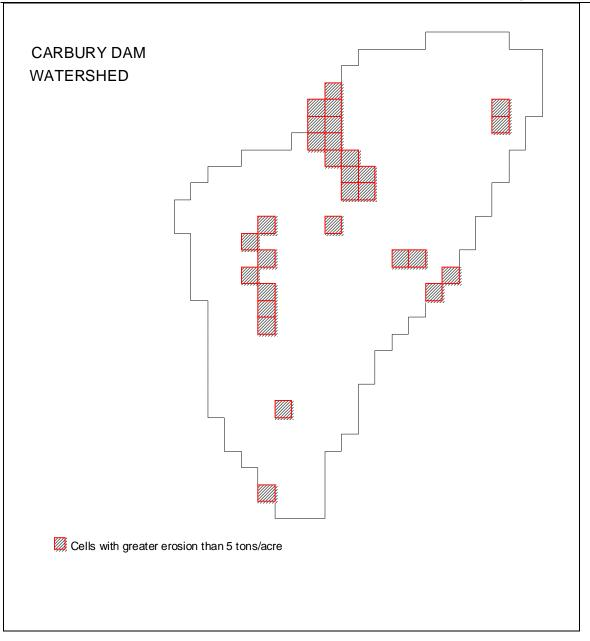
Figure 20. Cells within Carbury Dam Watershed with Soil Erosion > 5 tons/ac.
